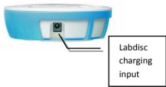
The **Labdisc** charger will accept any input voltage ranging from 100 to 240 VAC 50/60 Hz, making it functional worldwide.
